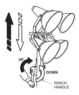
Figure 18. Adjusting Height of Light
